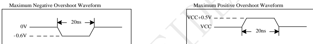
Figure 5-2 Input Test Waveforms and Measurement Level
